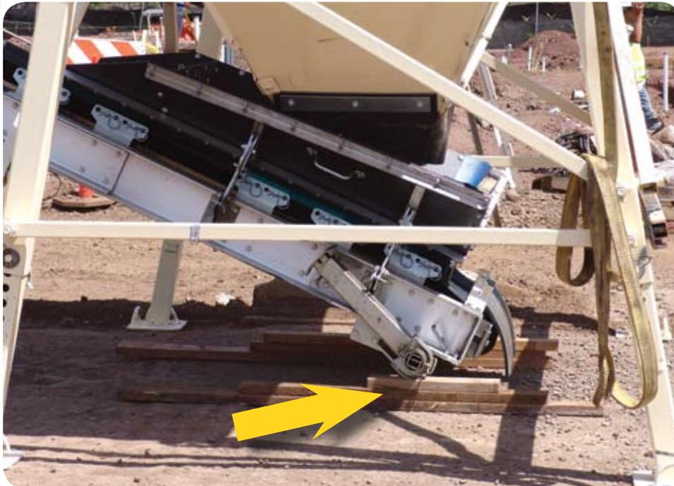
For a better hopper-to-hopper fit, your feed conveyor needs a boost off the ground when it's working with the standard folding Telebelt hopper. Just fold up the feed conveyor's legs and set the conveyor bottom on blocks or wooden planks instead of just placing it directly on the ground (see diagram). This is important in preventing the tail pulley under the hopper from being exposed to and damaged by rocks. Plus, it makes a better fit for discharging materials between hoppers.
